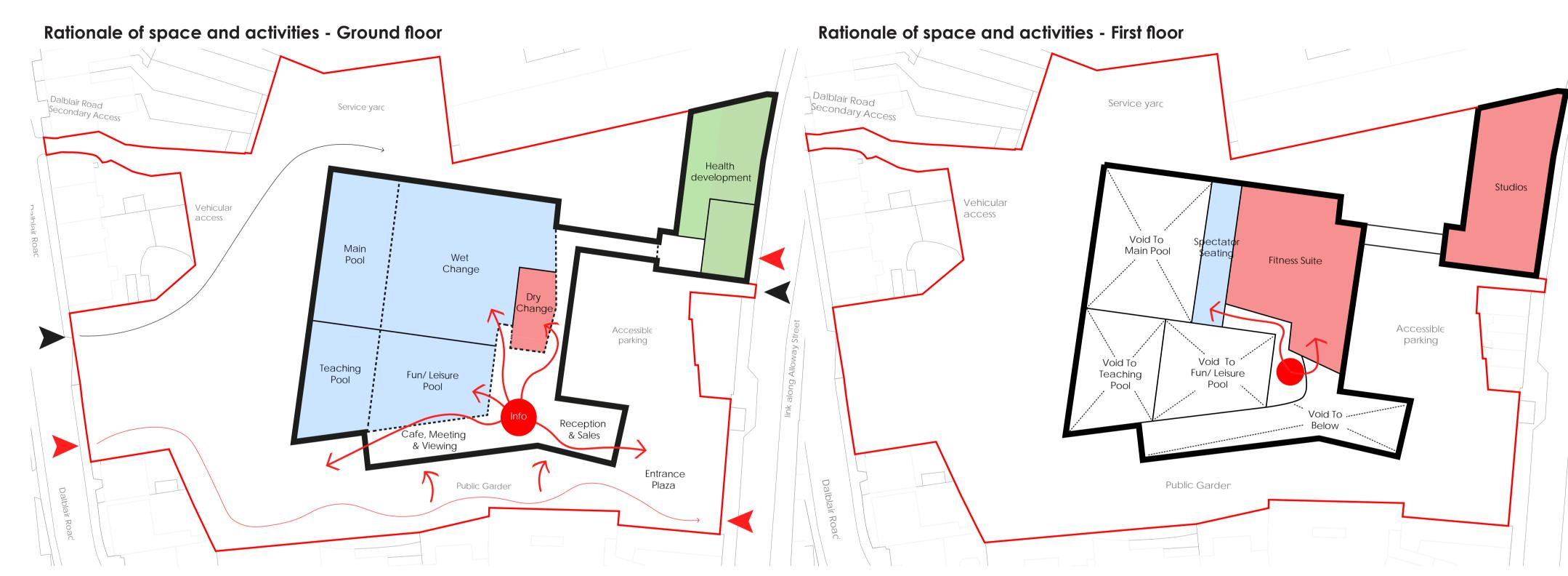
The diagram of the ground floor. A central foyer will allow access and views into all parts of the building and out into the proposed public garden and new entrance public
